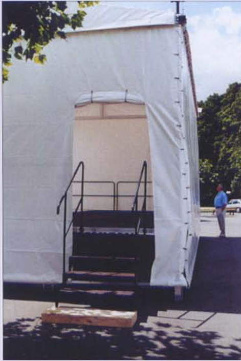
Door within the side-canopy and stair (stickable) with balustrade.
